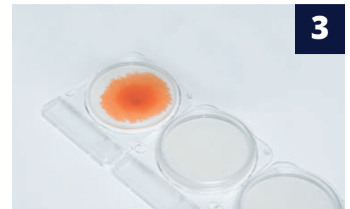
The sample diffuses passively and evenly across the dehydrated media sheet, rehydrating the dry medium into a gel within seconds.
