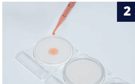
Dispense 1 ml of sample in the middle of the Compact Dry plate.
