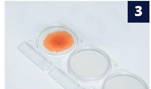
The sample diffuses passively and evenly across the dehydrated media sheet, rehydrating the dry medium into a gel within seconds.
