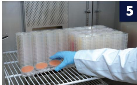
Turn over the plate (lid down) and incubate for the appropriate time and temperature.
